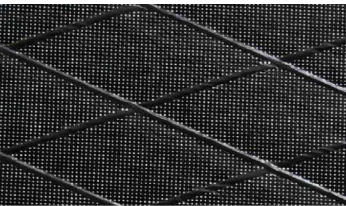
Magnified view of internal 100% Dyneema weave in S2Maui's ULTRA-HMPE™
